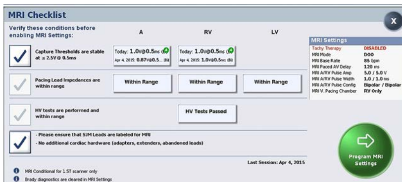
Figure 6. An example of the MRI Checklist screen for CRT-Ds on the Merlin PCS
