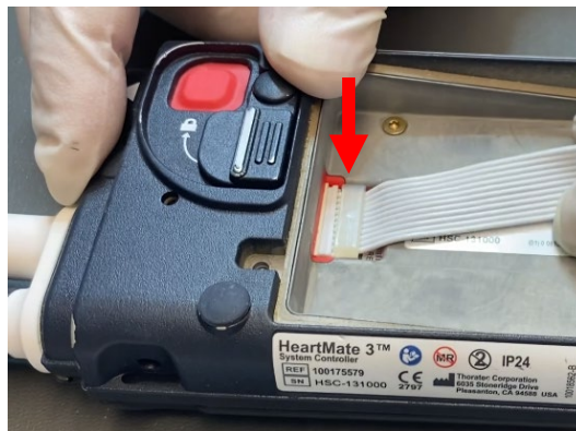
Figure 1: Connection of Backup Battery Ribbon Cable
