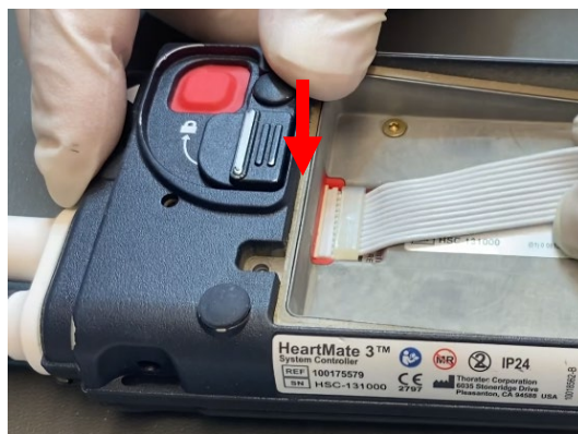
Figure 1: Connection of Backup Battery Ribbon Cable
