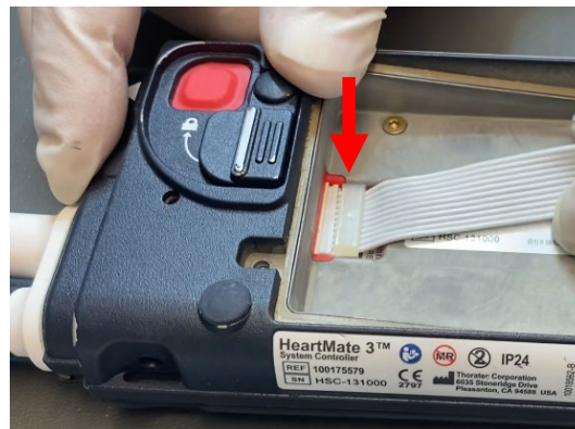
Figure 1: Connection of Backup Battery Ribbon Cable
