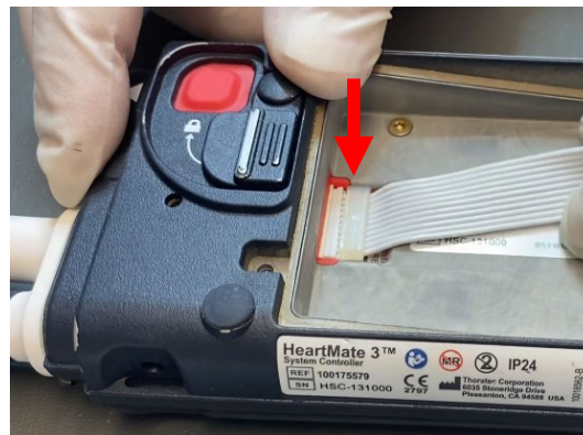
Figure 1: Connection of Backup Battery Ribbon Cable
