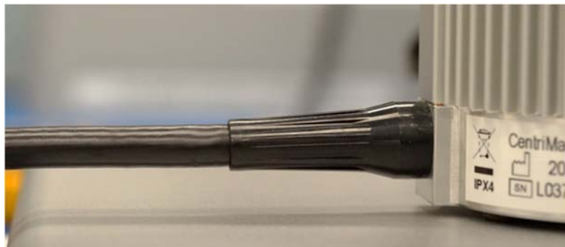
Figure 4: Cable Bend Relief at the Motor
