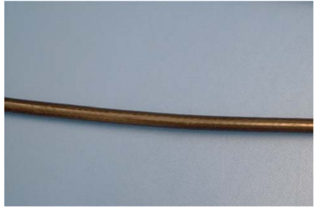
Figure 6: Undamaged and Intact Motor Cable
