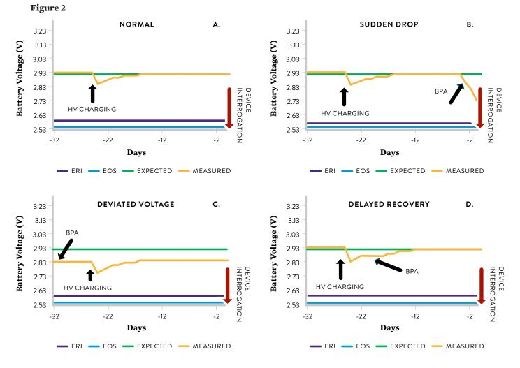
**Figure 2:** Examples of a normal BV trend (Panel 2a) and each of the patterns that the BPA will detect. The BPA arrow indicates the earliest detection point in each case.
