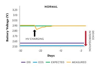
Three specific types of patterns were identified in the battery voltage trends that indicate that the battery is not performing as expected. The BPA algorithm was developed to trigger if these specific patterns are noted when comparing the measured battery voltage to the expected battery voltage.
