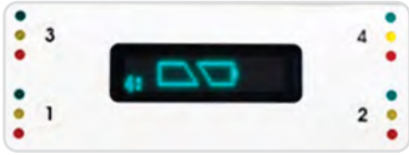
Calibration is in progress for 12 hours
