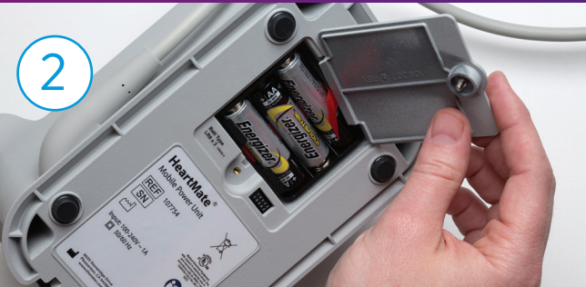
Open the battery compartment and pull the red ribbon to remove the batteries.
