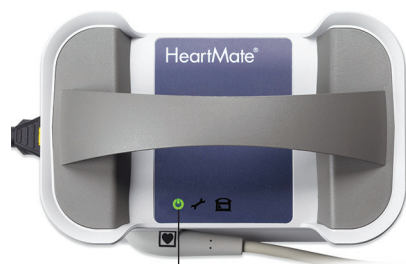
Normal: MPU power light is ON (green)
