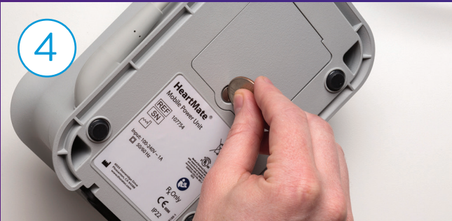
Close the compartment and tighten the screw.
