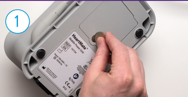
Loosen the screw from the rear panel.
