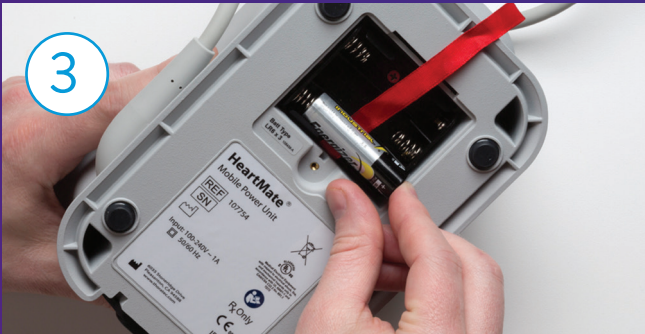
Place the alkaline AA batteries in the compartment.
