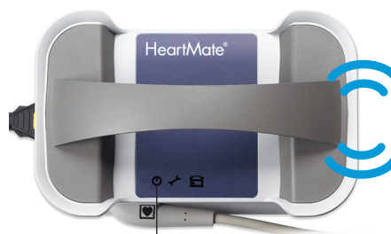
Damaged: MPU power light is OFF (black)
