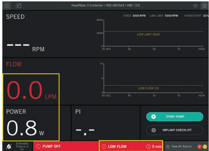
9. Access the **Pump** tab of the Settings panel and verify the fixed speed is set at 3,000 rpm and the low speed limit at 5,000 rpm. If not, enter the correct speed value, then tap **APPLY** if any change is made.
