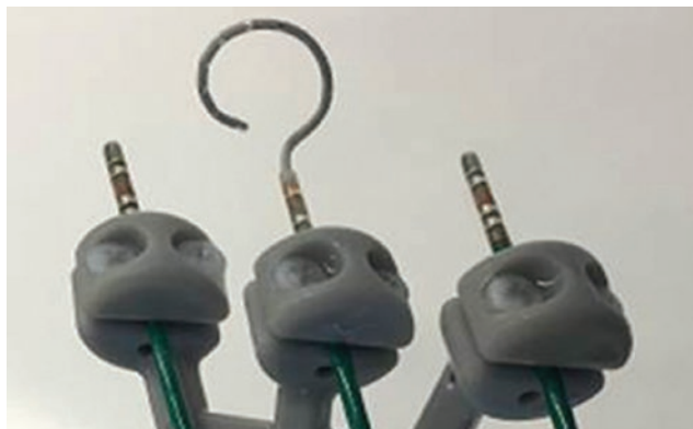
FIGURE 4: DWL fixture showing two FlexAbility™ ablation catheters, Sensor Enabled™ and one Advisor™ FL circular mapping catheter, Sensor Enabled™
