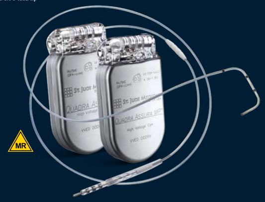
The Quartet<sup>™</sup> Family of LV leads offers more distal shape options including the Large-S, Small-S and the Double Bend and more total electrode spacing options including 40, 47 and 60 mm to offer not only successful CRT Implant but true quadripolar flexibility and options to help patient optimization.
