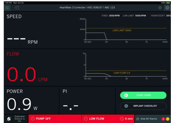
Figure 3: Clinical view after the completion of the “STOP PUMP” sequence.
