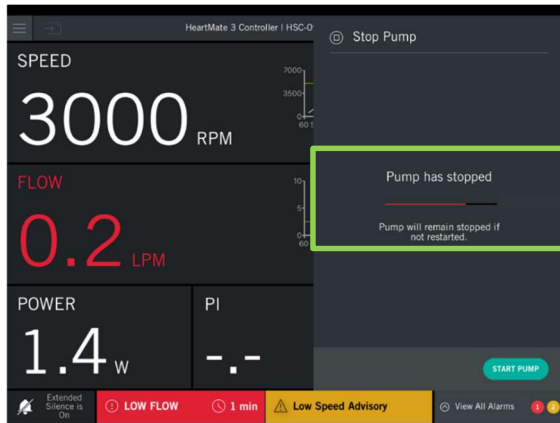
Figure 2: “STOP PUMP” red progress bar display on the black line indicating sequence is IN PROGRESS . Do not disconnect System Controller or Wireless Adapter.
