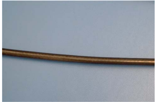
Figure 6: Undamaged and Intact Motor Cable
